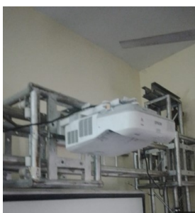
Figure 5. Side View of the Screen Projector Attached to Horizontal Dolly.
