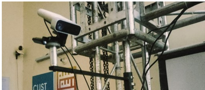
Figure 11. Left Sensor after Installation.
