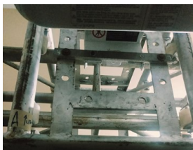
Figure 3. Fastening of the Screen Projector with the Horizontal Dolly.
